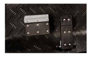
Press the upper section of the brake pedal until it locks in place to engage the parking brake. Press the service brake to release it.
