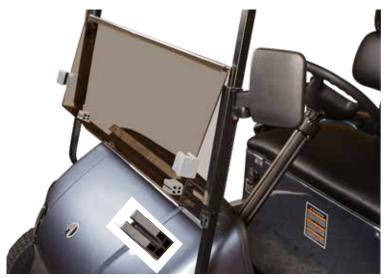
Slide the windshield rim into the rubber gaskets on both sides at the base of the windshield. Reverse the process to put the windshield back up.
