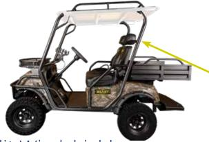
The canopy top provides protection from light rain and reduces exposure to sunlight. It will not provide shelter in heavy rain or protect you from falling objects and is not designed for roll over protection.
