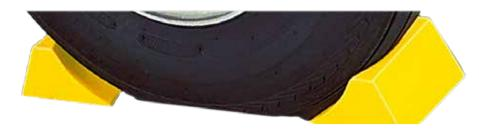
Place chocks in front of and behind both of the wheels on the end of the vehicle not being lifted.
