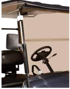
Carefully pry the rubber clamp at the top of the windshield from both sides of the frame.
