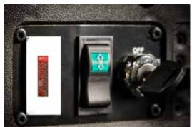
The top bar is illuminated when the batteries are fully charged.
