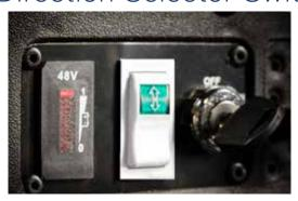
Press the three-position rocker switch to select the travel direction.
