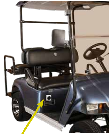
Charger receptacle located under the passenger seat
